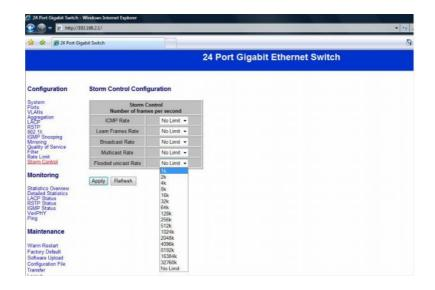
You can set up storm control by configuring the modes.
